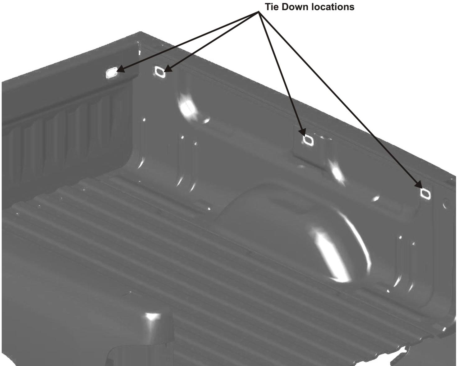
Step 2: Attach the 8mm bolt and 8mm threaded plate to the tie down as shown in the image below. With the plate towards the end of the bolt and in the rotated position as shown, insert the tie down assembly into the hole of the vehicle where the cover was removed.
