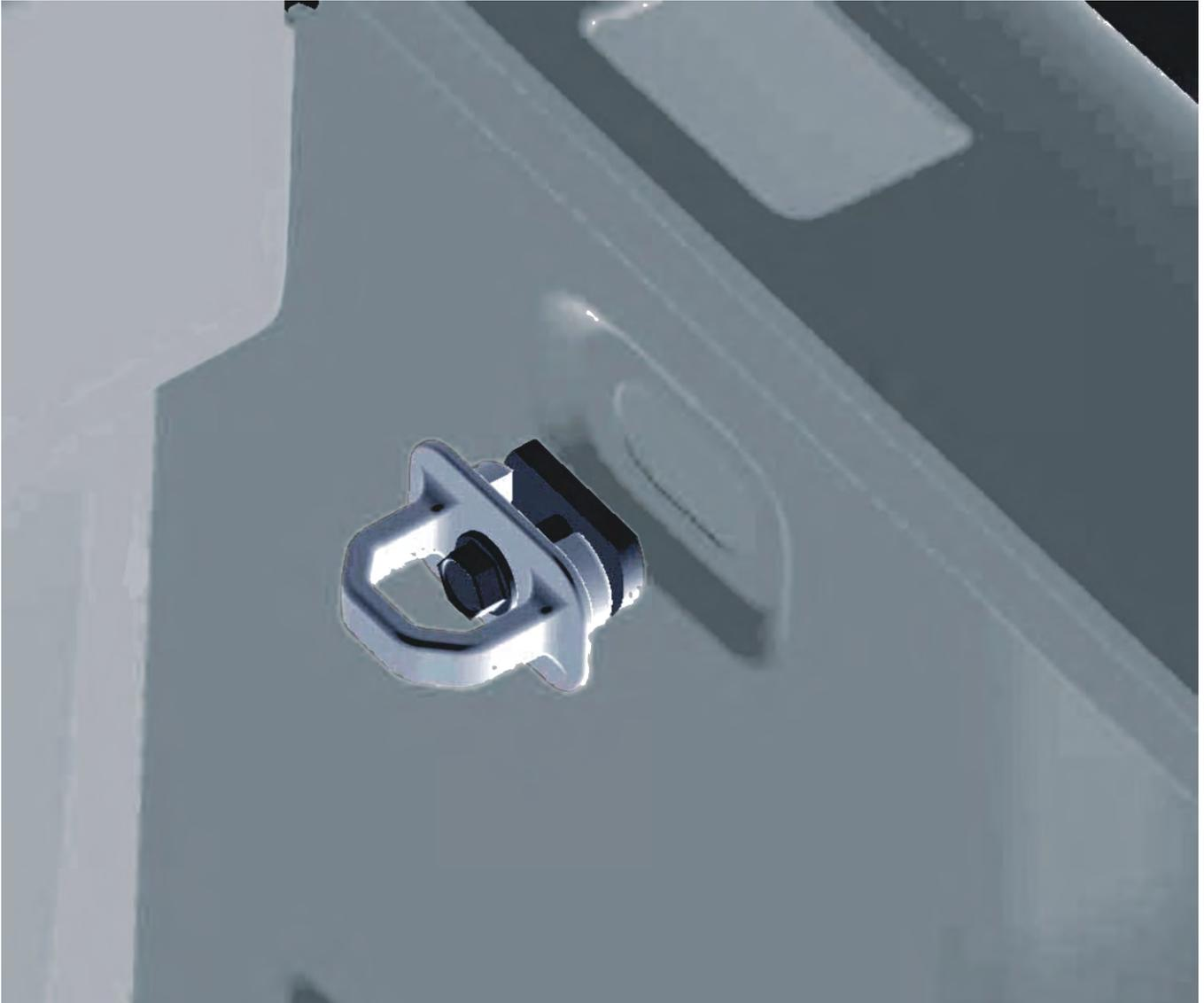
Tighten the bolt down by hand. Ensure that the plate has rotated in between the legs of the tie down to ensure a tight fit (refer to the image below). Once tight to the vehicle, torque the bolt down with a 13mm wrench to 16ft/lbs.
