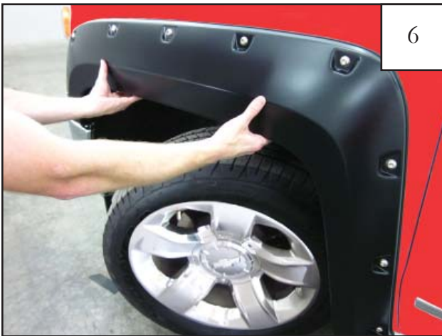
To mount the flare into position, hold the flare 2-3" inches below the top lip of the wheel well. Push in and slide up to allow flare to fully seat against the wheel well opening.
