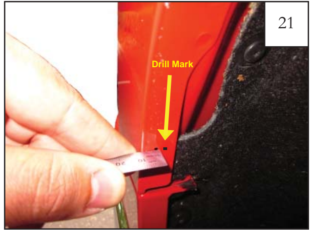
Remove the flare. Using the marks made in step 18 as a guide, measure inward from the outside edge of the fender to verify proper depth of original marked location. Mark must be minimum of 22mm in from outside edge of fender, if short, adjust marks to 22mm.
