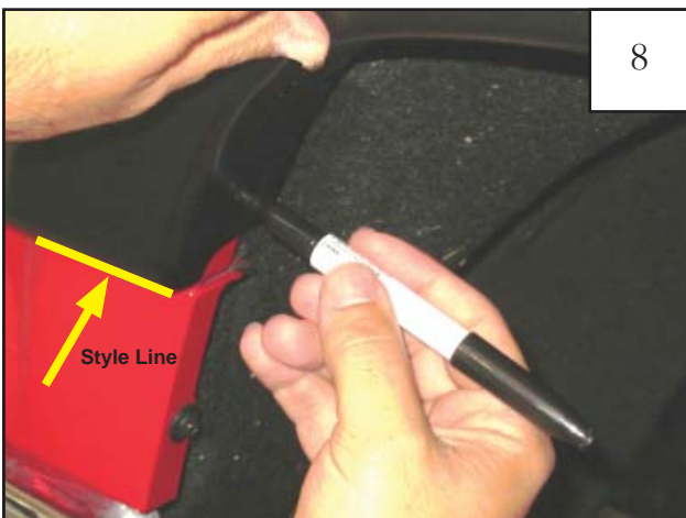
Hold front of the flare firmly on the fender. Make sure front of flare is aligned with bumper style line. Using a grease pencil, mark five hole locations using the holes in the flare as a guide. See next step.
