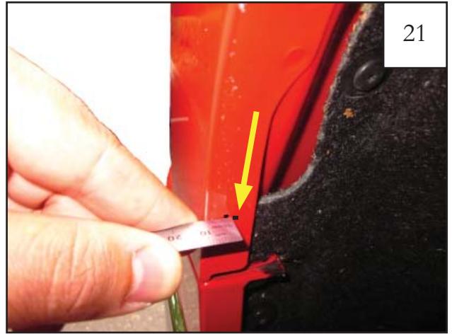
Remove the flare. At the marked locations made in Step 18, measure inward 22mm from the edge of the fender. These are the marks to be drilled. Note: Marks at 22mm may be on either side of the first mark.
